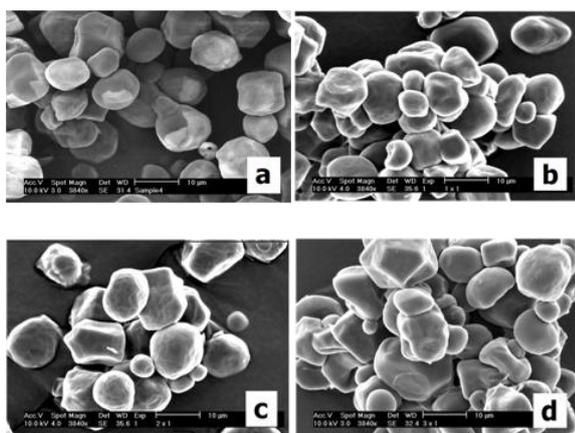
Fig. 1. Scanning electron micrographs of native and acetylated corn starches: (a) NCS, (b) ACS 160, (c) ACS 260, and (d) ACS 360 (Bars = 10  $\mu\text{m}$ ).
